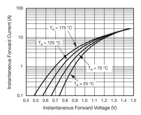
Fig. 3 - Typical Instantaneous Forward Characteristics
