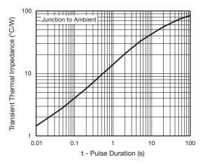
Fig. 6 - Typical Transient Thermal Impedance
