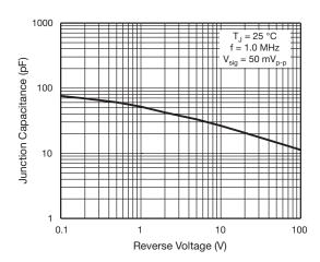
Fig. 5 - Typical Junction Capacitance
