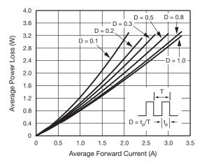
Fig. 2 - Forward Power Loss Characteristics
