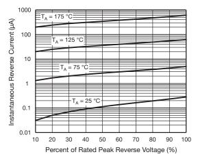
Fig. 4 - Typical Reverse Leakage Characteristics
